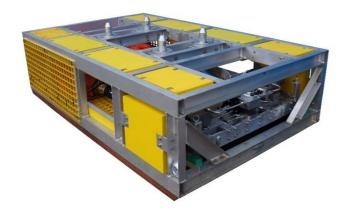
The image on the left shows our BOP Shutdown System mounted into a Multipurpose ROV skid as a package (RQ-037).
